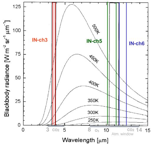
Figure.1. Plank Function and the location of AVHRR channel 3 and 4 and INSAT-3D Channel 3, 5 and 6
