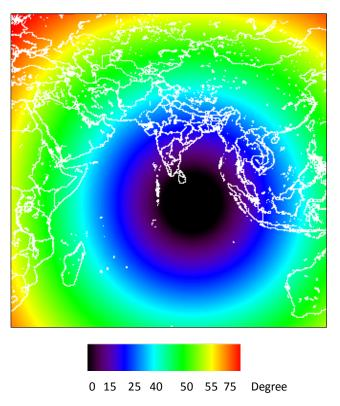
Figure 2. View zenith angle for the INSAT-3D satellite located at 84 degree E
