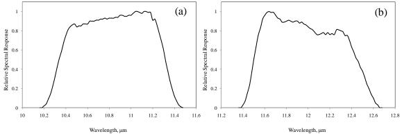
Figure 1. Spectral response functions two thermal infrared bands of INSAT-3D *Imager* (a) TIR1: 10.3-11.3 µm and (b) TIR2: 11.5-12.5 µm
