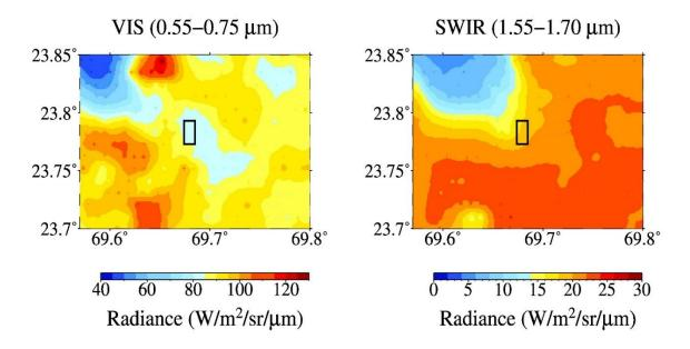
Figure 5: TOA radiance as observed by INSAT-3DR in its VIS and SWIR channels
