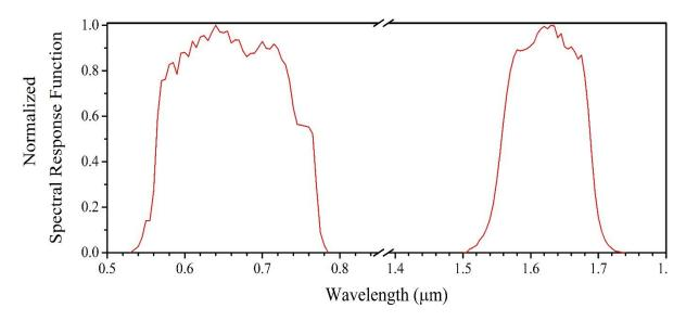
Figure 4: Pre-launch laboratory measurements of spectral response function for VIS and SWIR bands of INSAT-3DR
