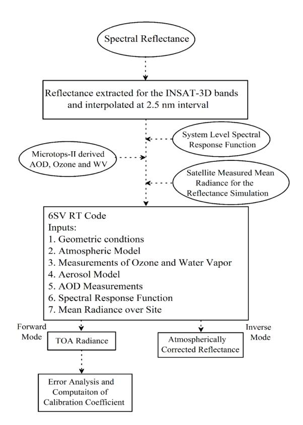
Figure 3: Detailed flow chart for the estimation of TOA radiance.
